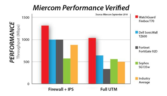
The HTTP throughput results, shown in the chart, reveal the variability between security appliances as more and more security functions are enabled.
